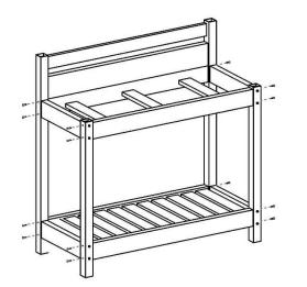
Using four ¾" screws per post, screw together potting bench. Be sure that all parts are fully inserted into posts before securing.
