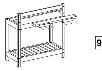
From behind, slide shelf through gap in back panel of potting bench. Using six  $\frac{3}{4}$ " screws, fasten wide end of brackets to  $1\frac{1}{2}$ " x  $5\frac{1}{2}$ " x  $46\frac{1}{2}$ " back rail. Snap kappet screw caps over screw heads.
