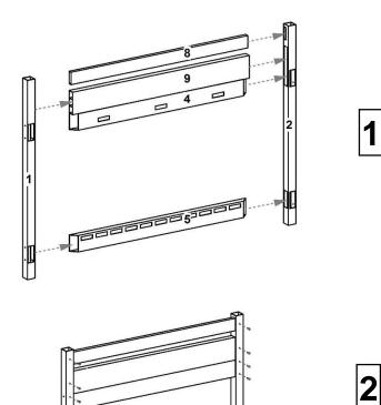
Insert  $\frac{7}{8}$ " x 3" x 46½" back rail (part 8) into top hole in back right post (part 2). Insert 1½" x 5½" x 46½" back rail (part 9) into top of large hole of back right post. Insert one table support (part 4), into bottom of large hole of back right post. Insert one shelf support (part 5) into bottom hole of right back post. Insert free ends of all rails into corresponding holes of back left post (part 1).
