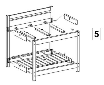
Insert three  $\frac{7}{8}$ " x 3" x 20 $\frac{7}{4}$ " table/shelf rails (part 7) into table support of back panel. Insert eleven  $\frac{7}{8}$ " x 3" x 20 $\frac{7}{4}$ " table/shelf rails (part 7) into shelf support of back panel. Insert two 1 $\frac{7}{4}$ " x 4" x 20 $\frac{7}{4}$ " side rails (part 6) into back right and back left post. Insert free ends of all rails into corresponding holes of front panel.
