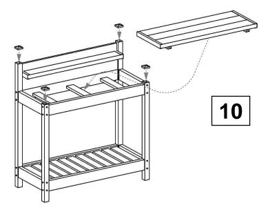
Apply PVC glue to inner edges of four 2" sq. post caps and place on top of each post. Set table top assembly into working area of potting bench. The table top is designed to be removed for easy and quick cleaning.
