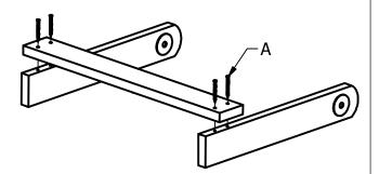
**3)** Attach Back Support Brace (shorter piece) to Back Support Sides with four A screws.
