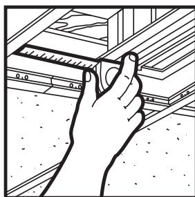
To install around obstructions, such as a post or vent, draw its exact location on the panel and make the cutout with a utility knife. To slide a panel over pipes, cut to opposite sides and install panel in two pieces.
