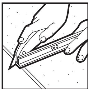
To cut a panel, place it on a flat surface, finished side up.
