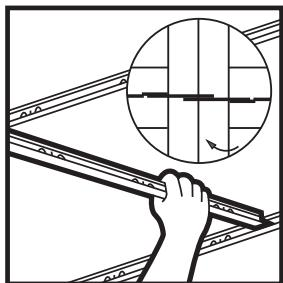
**11. Install cross tees** — After main tees are hung, install cross tees. Push cross tee end through the main tee slot until you hear a "click." Where two cross tees intersect in the same slot, be sure to insert the second tee to the left of the first.
