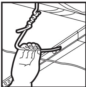
**10. Hang main tees** — Pull each hanger wire through the hanger hole in the tee. After checking the string line to be sure the tee is level, bend the wire up and around itself several times to ensure a good, tight wrap.
