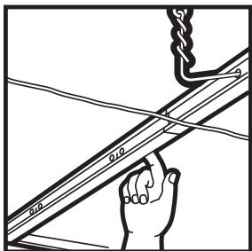
**9. Align first main tees** — In each row, trim the first main tee at the wall so that the slot for the first row of cross tees lines up at the string. Rest the cut end of the main tee on the wall angle.
