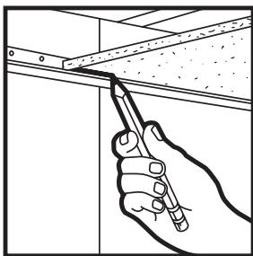
Trimming for shadow line edge: After cutting panel to size, fit it into the grid with cut edge against the wall. Draw a line on face of panel where it intersects wall angle. On the line, make a face cut to match depth of shadow line recess. Then, cut in from the panel edge to trim to proper depth.
