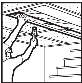
If a window or stairwell extends above the ceiling plane, build a valance with 3/4-in. (19 mm) lumber. Fasten it to walls and joists or to the old ceiling. Attach wall angles to the valance as you would to walls.
