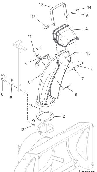
SERVICE PARTS: 52005600 - DISCHARGE CHUTE W/ CAP AND DECAL
