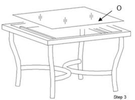
Important: please do not tighten any screws until all the screws are in the right position.
