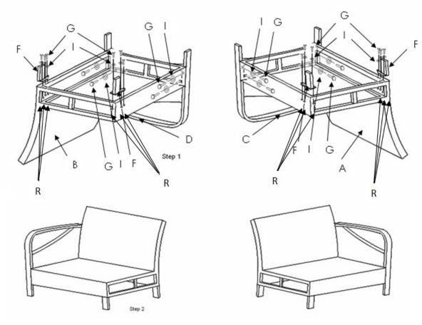
Important: please do not tighten any screws until all the screws are in the right position.
