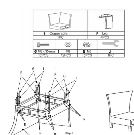
Important: please do not tighten any screws until all the screws are in the right position.
