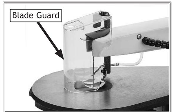
Figure 33. Blade guard position example.
