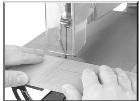
Figure 19. Example of making a straight cut.
