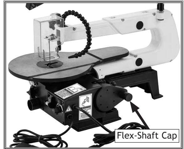
Figure 12. Flex-shaft cap location.
