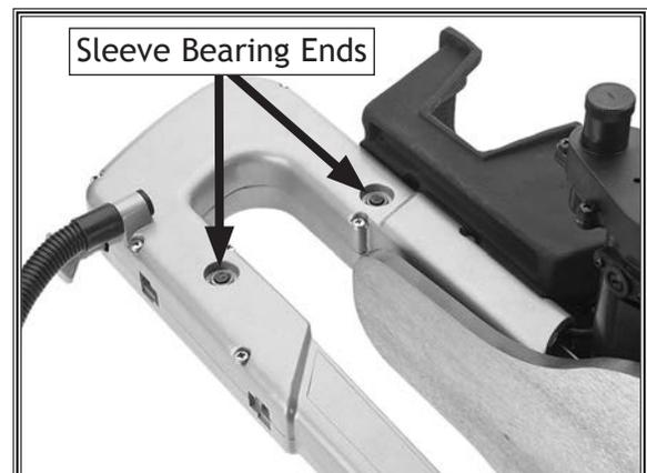
Figure 34. Plastic caps removed to expose sleeve bearing ends.
