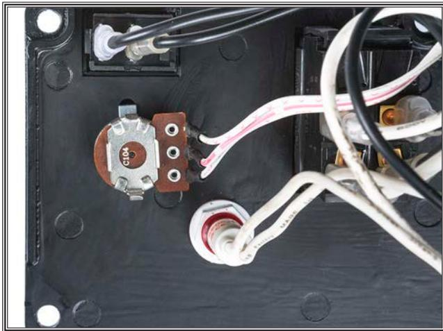
Figure 43. Foot pedal switch & potentiometer.
