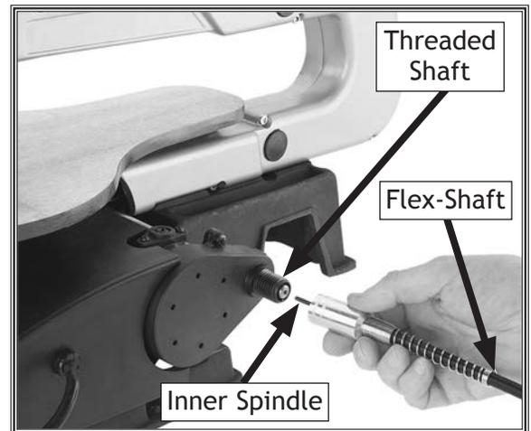
Figure 13. Example flex-shaft installation.
