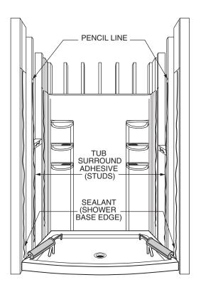
**C)** Align the top nailing flange of each side panel with pencil line marked. Press firmly into place to ensure proper adhesion to studs.
