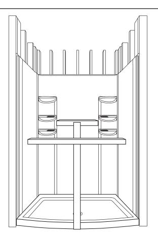
When installing greenboard, position drywall screws above the top nailing flange. If you choose to screw through the nailing flange, you MUST drill clearance holes in the flange to avoid cracking/damaging the flange.
