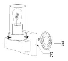
5. Attach the mounting plate (B) to outlet box with mounting screws (D)
