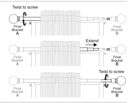
While holding the thickest tube, twist the middle tube away from you to lock it into place (as indicated by directional sticker). Twist until tight.
