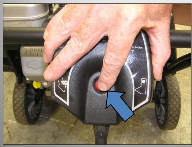
Depress the starter push button. After you start the engine, first disconnect the extension cord from the wall receptacle and then from the power cord receptacle.
