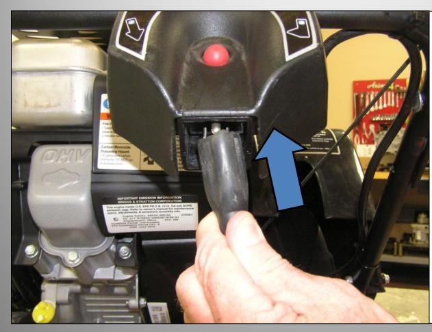
First connect the extension cord to the power cord receptacle and then into a wall receptacle. If additional extension cord is required, make sure it is three-wire.
