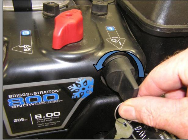
Before stopping the engine, allow it to idle for a few minutes to help dry off any moisture. Turn the ON/OFF key to the OFF position and remove key.
