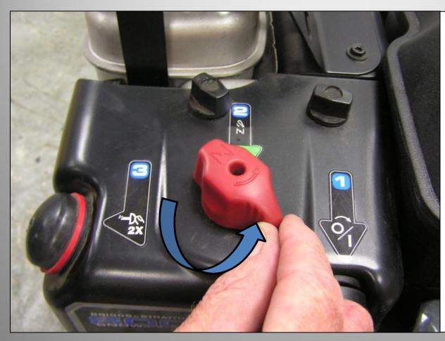
Turn the choke knob fully clockwise if engine is cold.
