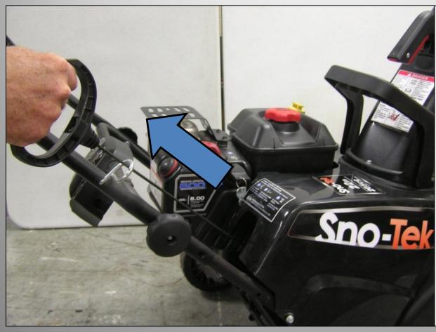
Firmly hold the starter cord handle. Pull the starter cord handle slowly until resistance is felt, then pull rapidly.
