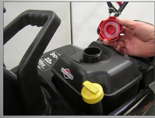
Fill the fuel tank with fuel. To allow for expansion of the fuel, do not fill above the bottom of the fuel tank neck. See Owners Manual for acceptable fuel.
