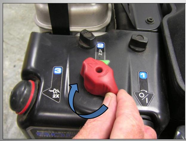
Allow the engine to warm up for several minutes, Then, slowly move the choke control knob to the run position.
