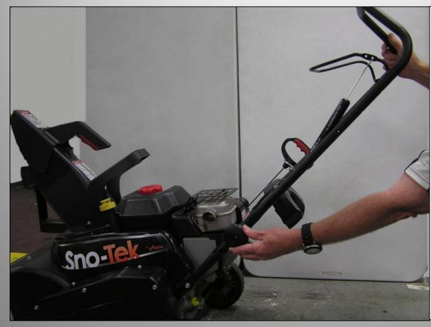
Loosen knobs on both sides of handle. Rotate the handlebar into operating position and tighten the knobs.
