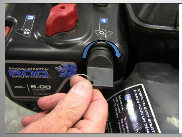
Insert the ON/OFF key and turn to the ON position.
