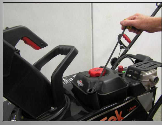
**NOTE**: The engine was shipped from the factory without oil. Before you start the engine, make sure you add oil according to the instructions in your Owners Manual. If you start the engine without oil, it will be damaged beyond repair and will not be covered under the warranty.
