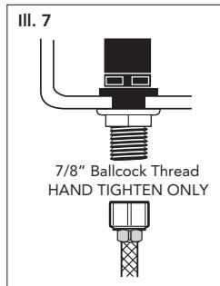
**CAUTION:** Avoid using a wrench to tighten the connection as you may damage the plastic threads and/or cause the fill valve to rotate inside the tank.
