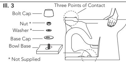
**CAUTION:** Do not over-tighten the nuts as damage to the china bowl may result.
