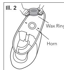
**CAUTION:** Do not move the bowl after the bowl wax ring is set. Thread the nuts and tighten evenly until bowl is snug to closet flange. Install the bolt caps (see Illustration 3).
