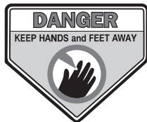
Figure B: Safety Label Found On Lawn Mower: KEEP HANDS AND FEET AWAY FROM MOVING PARTS.
