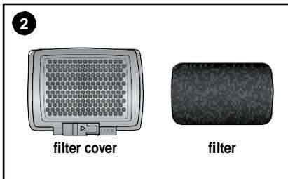
Remove filter cover with filter. Wipe with cloth over garbage bin, removing dirt and debris.
