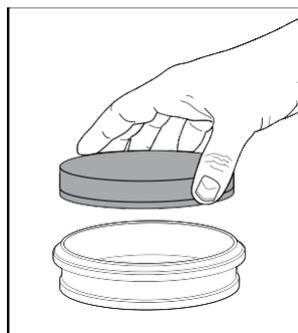
5. Allow filter to dry 24 hours before putting back into vacuum cleaner.
