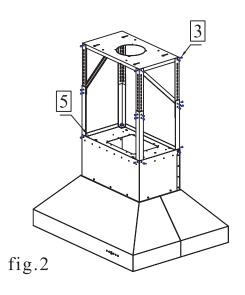
Step three: Take the chimney sections and separate slightly to reveal the vent slots. Next take the hood and slide the top mounting bracket over the mounting screws and slide back into position. fig 3. Make your electrical and duct connections at this point using 8 inch rigid ducting wherever possible.
