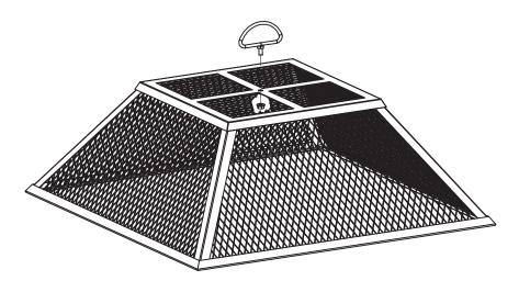
**Step 1:** Connect Handle (A) and Mesh Wire Cover (B) by using Nut M6 (H) and tighten with wrench.
