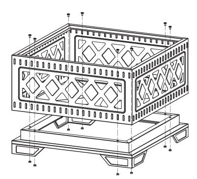
**Step 3:** Contact the Fire Bowl (C) with the Base (D) by using Bolt (G).
