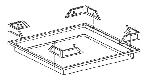
**Step 2:** Turn over the base (D) and contact it with Leg (E) by using Bolt (G).
