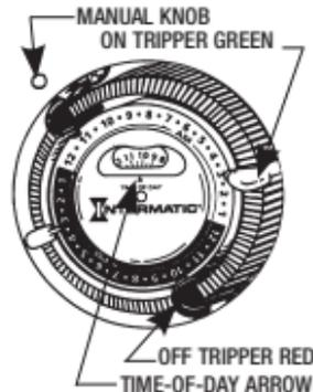
1. Insert **ON (GREEN)** and **OFF (RED)** trippers into dial at desired **ON** and **OFF** times.
