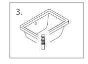
1. After installing the counter top on the cabinet, put the drain assembly inside the hole in the sink and fix it firmly.
