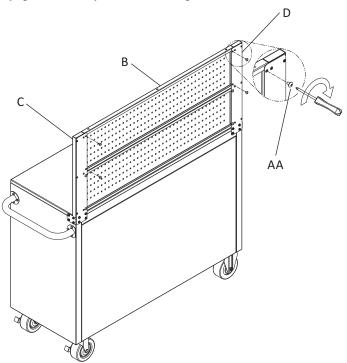
9. Ensure the front pegboard panels are flush. Using a Phillips-head screwdriver, tighten the three M6 screws (AA) to connect the bottom panel (A) and top panel (B) together.
