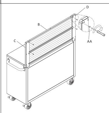
Ensure the front pegboard panels are flush. Using a Phillips-head screwdriver, tighten the three M6 screws (AA) to connect the bottom panel (A) and top panel (B) together.
