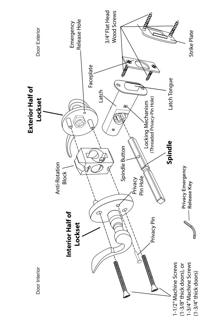
Exploded Drawing for Pre-Attached Rosette/Short Plates Passage/Privacy - Lever
