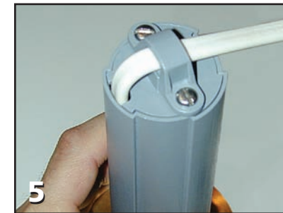
Figure 5 - Secure wire clamp on bottom of tube.
