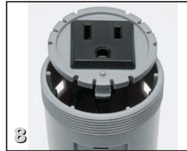
Figure 8 - Remove receptacle by pressing three tabs located on side of tube.
