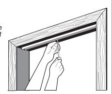
pre-drilled hole nearest the center of the track. Do not fully tighten. (Tape may be used to hold the track in place while you mark and drill.)
