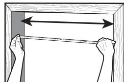
to alter the height of the door. If the opening is less than 80" high, the door may be shortened by sawing the excess from the bottom of the door panels.
