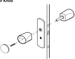
up with the screw shaft on the other side of the door. Tighten with screwdriver until secure.
