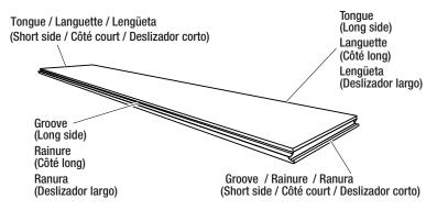
Lay out several cartons. Randomly rack planks to ensure good color and shade mixture and end joint spacing. Minimum end stagger is 6 in. Inspect plank quality and grading.
