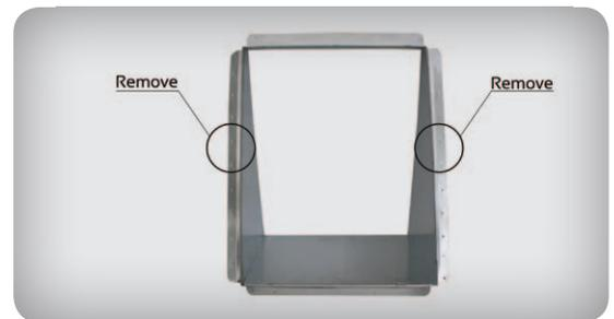
3. Using a flat head screwdriver, remove the two side flanges on the damper box. Make sure that you are removing the flanges on the same side as the flanges you removed on the vertical adapter. **(See Figure 2)**
