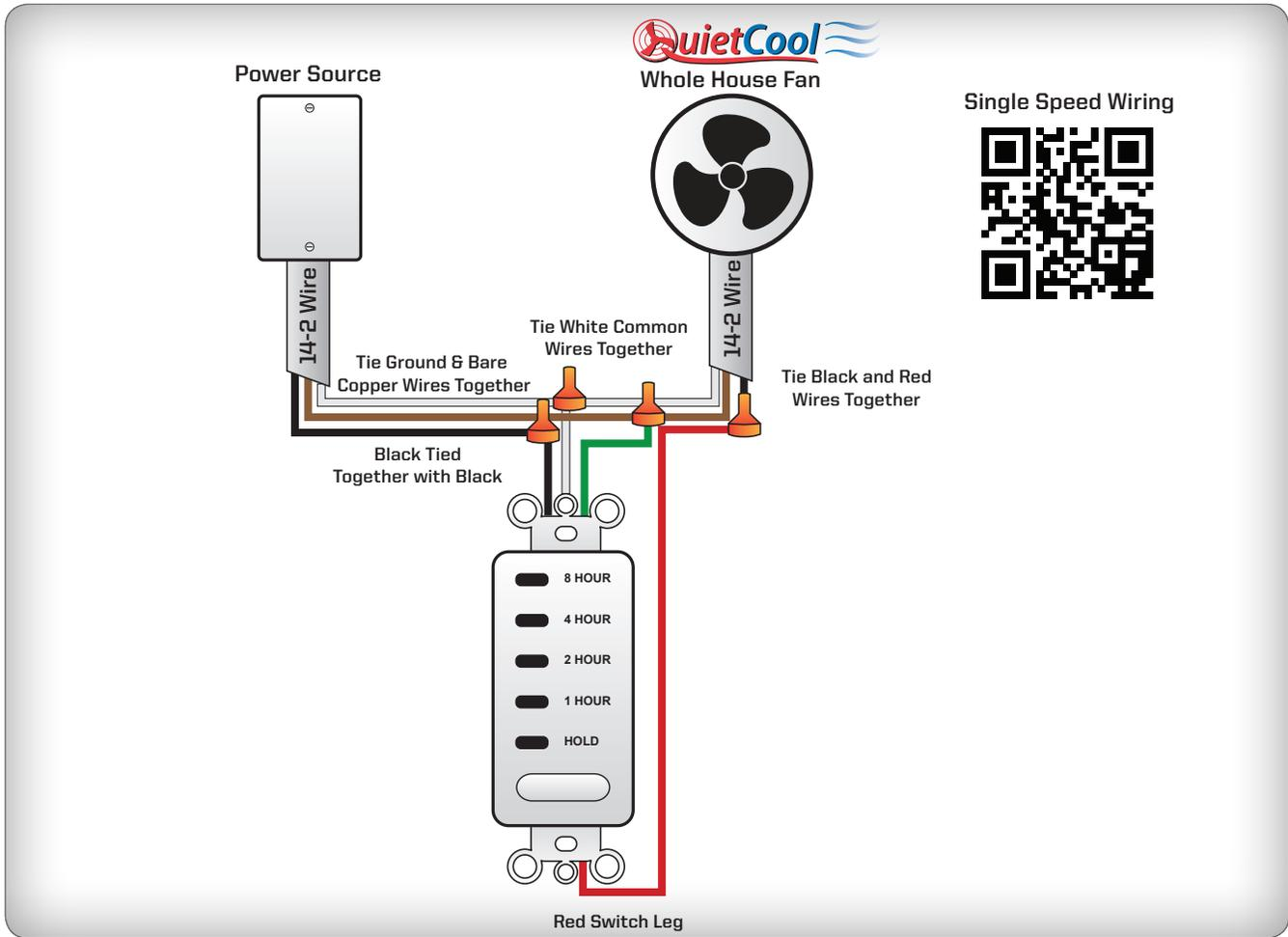
6. Feed the 2 wire Romex through the handy box. Using the included wire nuts, tie the black wires together. Tie the white neutral wires together. Tie your bare copper wire and green ground wires together.
