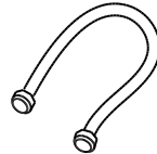
Toilet water supply line
