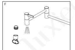
F. Remove aerator from the spout and turn on the water for about a minute to flush out any debris in the plumbing system. Also check for leaks at all connections. Re-install the aerator when done. This faucet is equipped with two on/off handles, the handle on the wall side should be closed (handle in vertical position) when faucet is not in use. If the pot filler is to be left unattended, please ensure both handles are in closed position.
