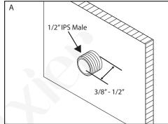
A. Shut off the main water supply before installation. The faucet requires an 1/2" IPS/NPT threaded male nipple extending 1/2" from the finished wall. For ease of future maintenance, it is recommended to install a shut off valve for the water supply line at an easily accessible location.
