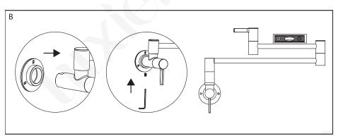
B. Place mounting base (19) onto pot filler body (15). Attached the assembly onto the nipple on the finished wall surface and secure the setscrew (22) to hold the faucet in place. Do not fully tighten the setscrew. Use a level to make sure the faucet is level and plumb. Use a marker to mark 3 positions for drilling. (NOTE: Make sure there are no pipes or electrical wires behind the mounting surface.)
