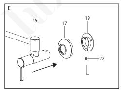
E. Slide the flange (17) onto the faucet body (15) first and attach the faucet to the male threaded nipple. Once the faucet is attached to the pipe tighten the setscrew (22) and slide the flage to cover the mounting base (19)
