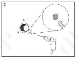
C. Remove the faucet from the wall and use a power drill to drill the 3 holes needed for installation. Insert wall anchors into the holes when done. Apply TPFE tape onto the nipple in counterclockwise direction.
