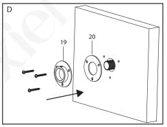
D. Place the rubber gasket (20) onto the wall and attach the mounting base (19) with the included screws. Loosen the setscrew (22) on the mounting base. (NOTE: Make sure the rubber gasket and the mounting base securely attached to the wall to prevent water from entering the wall cavity.)
