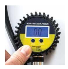
Press the UNIT button to switch between modes.
