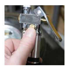
Press the Bleeder Valve to inflate. Releasing it will also reset the device.
