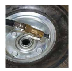
Use the Closed Flow Air Chuck to inflate/deflate tires. The closed flow design allows air to flow when the internal flow valve is open.
