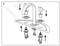
F. Insert hot and cold valves from underneath the mounting surface. Secure the handle assemblies with the decorative trims from top of the mounting surface.
