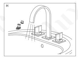
H. Use the aerator wrench to remove the aerator. Turn on both hot and cold handles and let the water run for about 1 minute to flush out any sediment or debris inside the plumbing. Also check for leaks at all connections.
