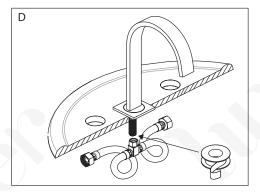
D. Apply Teflon (TPFE) tape on the thread of the center spout brass pipe. Use an adjustable wrench to tighten the fittings. (NOTE: Do not overtighten the connection.)
