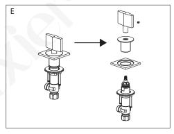
E. Use a small hex wrench to loosen the small setscrew on the handle. Lift up the decorative trim handle and remove all trim pieces.
