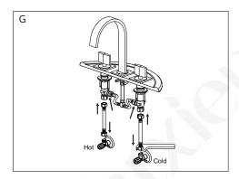
G. Apply Teflon (TPFE) plumbing tape on both valve assemblies and shutoff valves. Attach water supply hoses with 1/2" fittings (not included) with an adjustable wrench. Also connect the water hose between the handle assemblies and the center spout. (NOTE: Do not overtighten the connection.)
