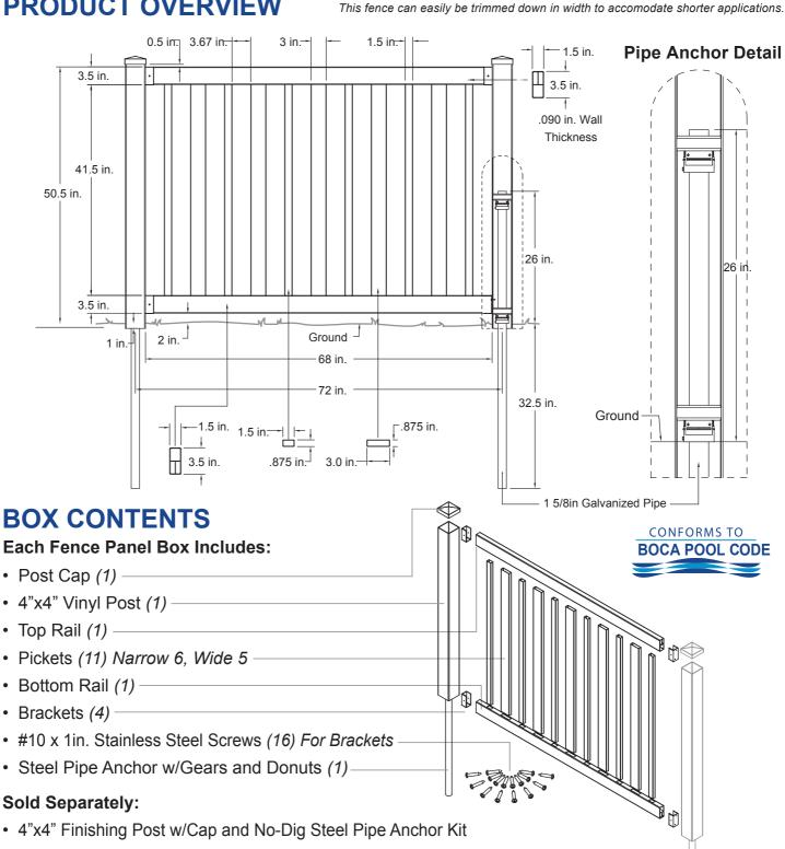
4"x4" Finishing Post w/Cap and No-Dig Steel Pipe Anchor Kit sold separately (see note on left)-
