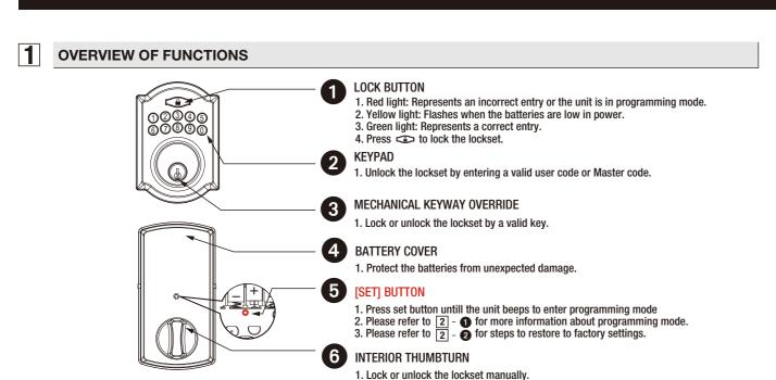
**HOW TO LOCK / UNLOCK THE LOCKSET** To lock Press " To lock. Use a mechanical key to lock. 0R Enter a valid User Code Use a mechanical key to unlock. or the current Master 0R Code to unlock
