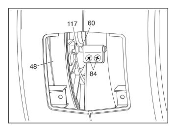
Next, rotate the Large Pulley (48) until a Pulley Magnet (117) is aligned with the Reed Switch (60). Slide the Reed Switch slightly toward or away from the Pulley Magnet. Then, retighten the M4 x 19mm Screws (84).
