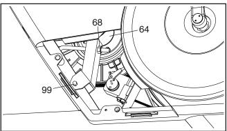
When the Drive Belt (64) is tight, tighten the M10 x 55mm Bolt (99). Then, reattach the side access cover.
