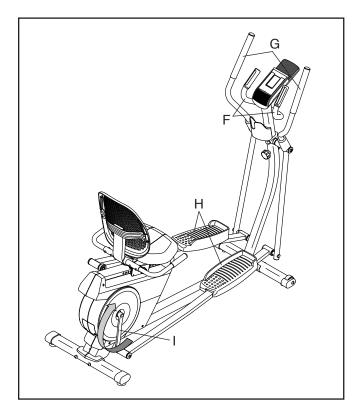
Push the pedals (H) until they begin to move with a continuous motion. Note: The crank arms (I) can turn in either direction. It is recommended that you move the crank arms in the direction shown by the arrow; however, for variety, you can turn the crank arms in the opposite direction.
