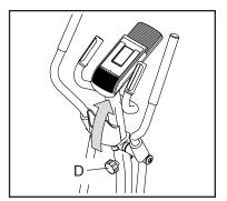
Then, lift a pedal, fold the brace (E) upward, and pivot the pedal downward to the low position. **Repeat this action for the other pedal.**
