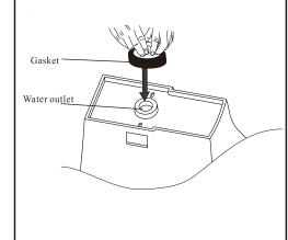
4. Flip water closet upright and gently set the toilet on the closet flange making sure to line up the T# screw closet bolts in alignment with the two holes at the base of the toilet. Firmly press the water closet towards the floor, until the water closet sits level on the floor.
