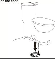
5. Install the spacer nuts and screw covers by accessing the T# screw closet bolts from the rear and side of the water closet. Tighten both sides by hand first, rotating from side to side until the water closet is snug and level against the floor. Next tighten with a wrench again, rotating side to side until the water closet is firmly set and level on the finished floor. DO NOT OVERTIGHTEN. Over tightening can cause the porcelain to crack, voiding product warranty.
