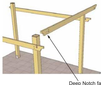
5. Locate Girder with **Deep Notch on Bottom** (C) and lift up between both completed Post/Girder Assembly's.
