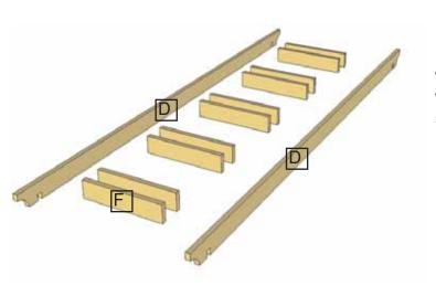
**12.** On a flat surface, position Ladder Blocking (F) where marked on top edge of Joist (D) and screw with 2 - 2 1/2" screws per end. Ladder Blocking should be flush with top and bottom of Joist with all notches facing down.
