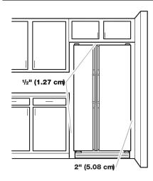
To ensure proper ventilation for your refrigerator, allow for 1/2" (1.27 cm) of space on each side and at the top. Allow for 1" (2.54 cm) of space behind the refrigerator. If your refrigerator has an ice maker, allow extra space at the back for the water line connections. When installing your refrigerator next to a fixed wall, leave a 2" (5.08 cm) minimum space on each side (depending on your model) to allow the doors to swing open.
