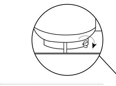
Remove the door panel (C) from the body (B) of the fire column and put the 20 lb. propane gas tank (not included) into the body (B). Turn the wing screw on the outside of the internal tank holder clockwise to tighten the tank into the holder.
