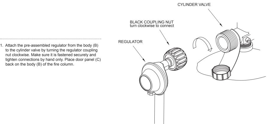
1. Attach the pre-assembled regulator from the body (B) to the cylinder valve by turning the regulator coupling nut clockwise. Make sure it is fastened securely and tighten connections by hand only. Place door panel (C) back on the body (B) of the fire column.
