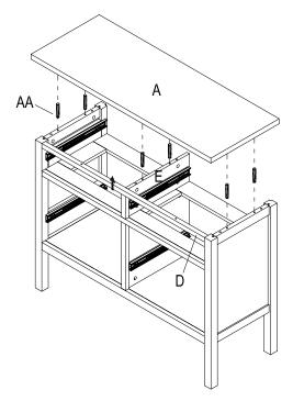
d) Tighten bolt (BB) with lock (CC) in the pre-drilled holes. Tighten bar (D) with screw (EE).
