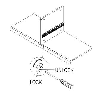
Wood dowel Cam lock bolt Cam lock Small head Large head
