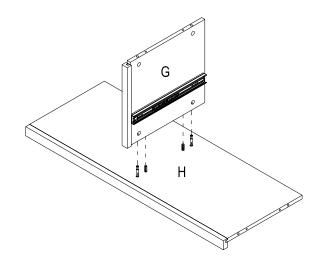
$\ \square$  d) Tighten bolt (BB) with lock (CC) in the pre-drilled holes.
