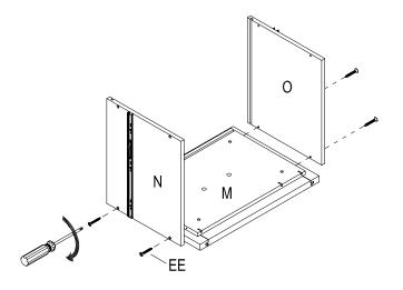
c) Tighten panel (P) to the assembled body with screw (EE).
