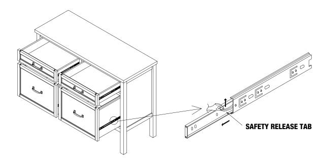
NOTE: When removing the drawer, tip-up the safety release tab to remove the drawer from the body.
