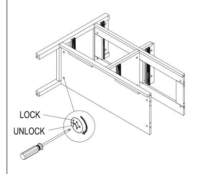
Wood dowel Cam lock bolt Cam lock Small head Large head
