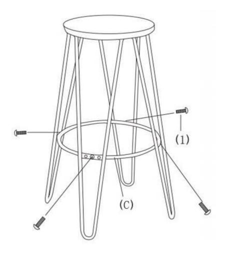
Attach Foot Ring (C) to Legs (A) with Allen Key Screws (1). Use Allen Key (2) to tighten all screws.
