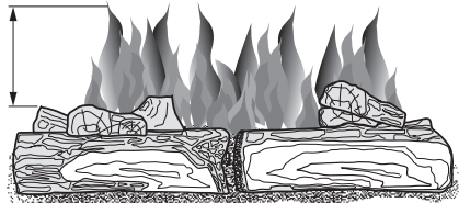
Figure 33 - Incorrect Burner Flame Pattern
