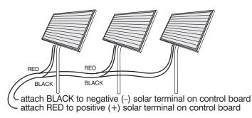
All connections should be made weatherproof using weatherproof splice kits available at hardware and electrical supply stores.
