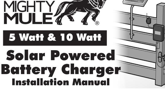
Compatible with GTO Access Systems and Mighty Mule DC Powered Gate Openers. NOTE: Dual gate installations require a minimum of 10 Watts of solar charging power.
