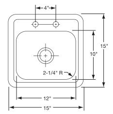
ALL DIMENSIONS IN INCHES, TO CONVERT TO MILLIMETERS MULTIPLY BY 25.4.
