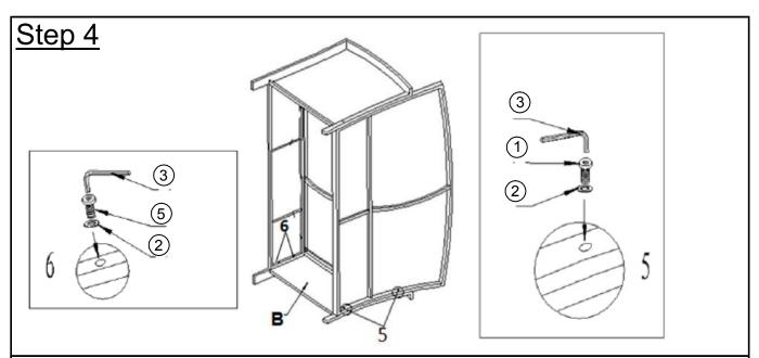
Place Left Armrest(B) against Backrest(K), Seat(L) and Front Panel(M). Attach the Left Armrest(B) to Backrest(K) using Hardware((1, 2)) with Allen Key((3)) as shown in Picture 5. Attach Left Armrest(B) to Front Panel(M) using Hardware((2, 5)) with Allen Key((3)) as shown in Picture 6. **Do not fully tighten the bolts at this stage.**
