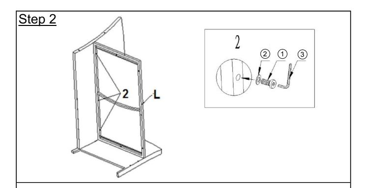
Place the Seat(L), as picture above so as to be attached to the Right Armrest(C) and Backrest(K) using hardware (1). 2) with Allen key(3) as shown in picture 2.
