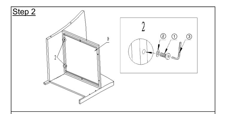
Place the Seat(D) between the Right Armrest(C) and Backrest(A). Attach Seat(D) to Right Armrest(C) using Hardware( 1, 2) with Allen Key(3). **Do not fully tighten the bolts.**
