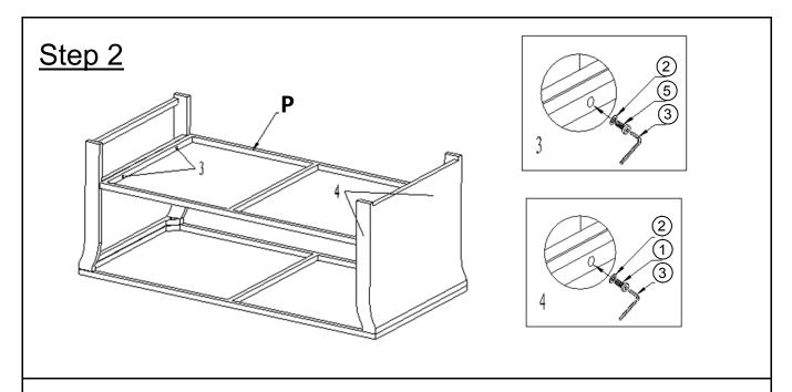
Attach the Table Shelf(P) between the two Table Legs(R) using Hardware ( $\mathfrak{S}$ ,  $\mathfrak{D}$ ) with Allen Key( $\mathfrak{S}$ ) as shown in Picture 3 and Picture 4.
