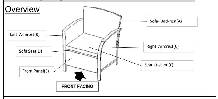
This Single Sofa has multiple parts and may require up to some 30 minutes to assemble. To give you an overview of the Single Sofa parts, the above picture is to help you put the various parts into perspective. Please read through the instructions herebelow to familiarise yourself with the parts and steps before assembly.
