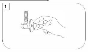
Shut off water supplies. Remove old faucet. Clean sink surface in preparation for the new faucet.
