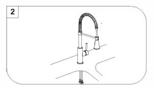
Place optional Flange on the bottom of the new faucet before positioning faucet through mounting hole.
