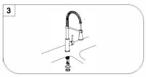
Screw the mounting stud into the body. Secure the faucet to the sink by installing steel washer and nut onto it. Tighten with wrench.
