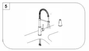
Important: After installation is completed. Turn on water supply and allow both hot and cold water to run for at least one minute each. While water is running, check for leaks. Reinstell Spray head. Your new faucet is now ready to use.
