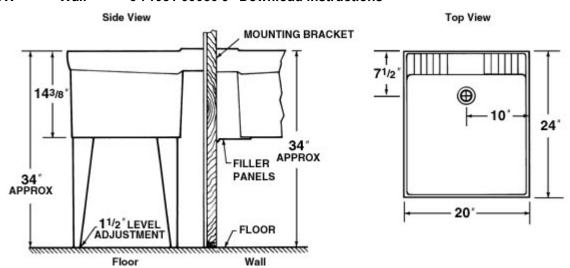
General: Furnish and install as shown on plans, UTILATUB® Laundry/Utility Tub model\_\_\_\_(19F, 19W), as manufactured by E.L. Mustee & Sons, Inc. Tub shall be one-piece molded construction using structural thermoplastic with matched metal molds under extreme heat and pressure. Tub to include integrally molded drain assembly, stopper and floor or wall mounting hardware. Shall meet ANSI Specification Z 124.6. White color. Weight: 19F 23 lbs.; 19W 20 lbs.
