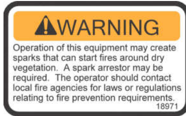
18971 - SPARK ARRESTOR WARNING
