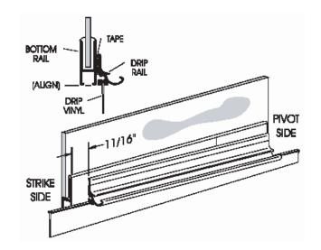
Adjust the drip vinyl [X] by sliding it left or right until it just touches the curb. Trim the vinyl (flush with the pivot end and notch 1/2" longer than the drip rail as shown on the strike end). Secure it with one #6 x 3/8" truss head screw [F] in the pivot end of the drip rail.
