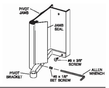
Place the pivot jamb assembly on the curb [A] with the exterior face lined up with the raised edge of the curb. Use a level to plumb the jamb then mark the mounting hole locations. Remove the jamb and drill the mounting holes.
