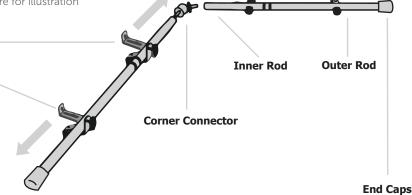
Ensure that that the rods are assembled as shown below:
