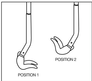
**NOTE:** Insert tool head fully under board for maximum lifting leverage.
