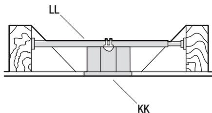
To hang your fan where there is an existing fixture but no ceiling joist, you may need an installation hanger bar (LL) (not included) as shown above.
