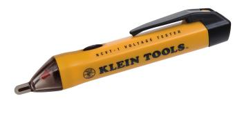
Use this Non-Contact Voltage Tester to detect standard voltage in cables, cords, circuit breakers, lighting fixtures, switches, outlets and wires. A bright green LED will tell you the tester is working and also functions as a worklight. It changes to red and warning tones sound when voltage is detected.
