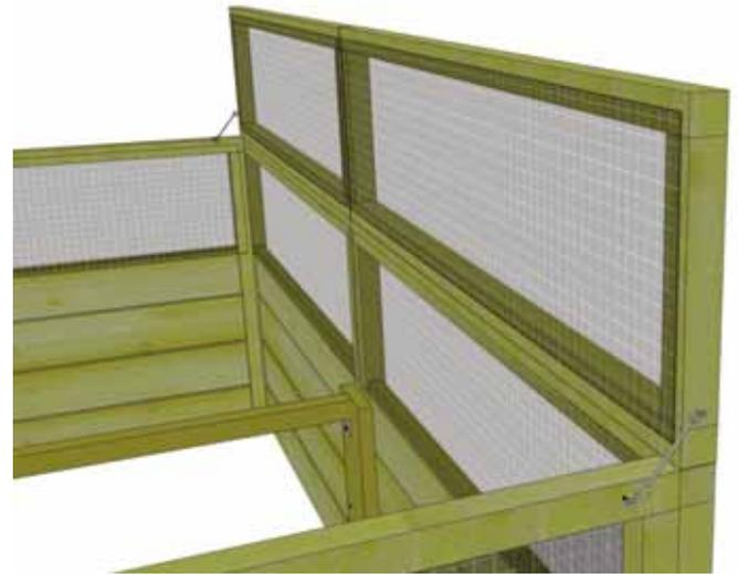
**25.** Lift trellis/screen into the up position. Screw male portion of **Eye Hook** into trellis/screen side framing and female piece into side framing of side wall. Do a dry run first to confirm correct position. Complete both sides.
