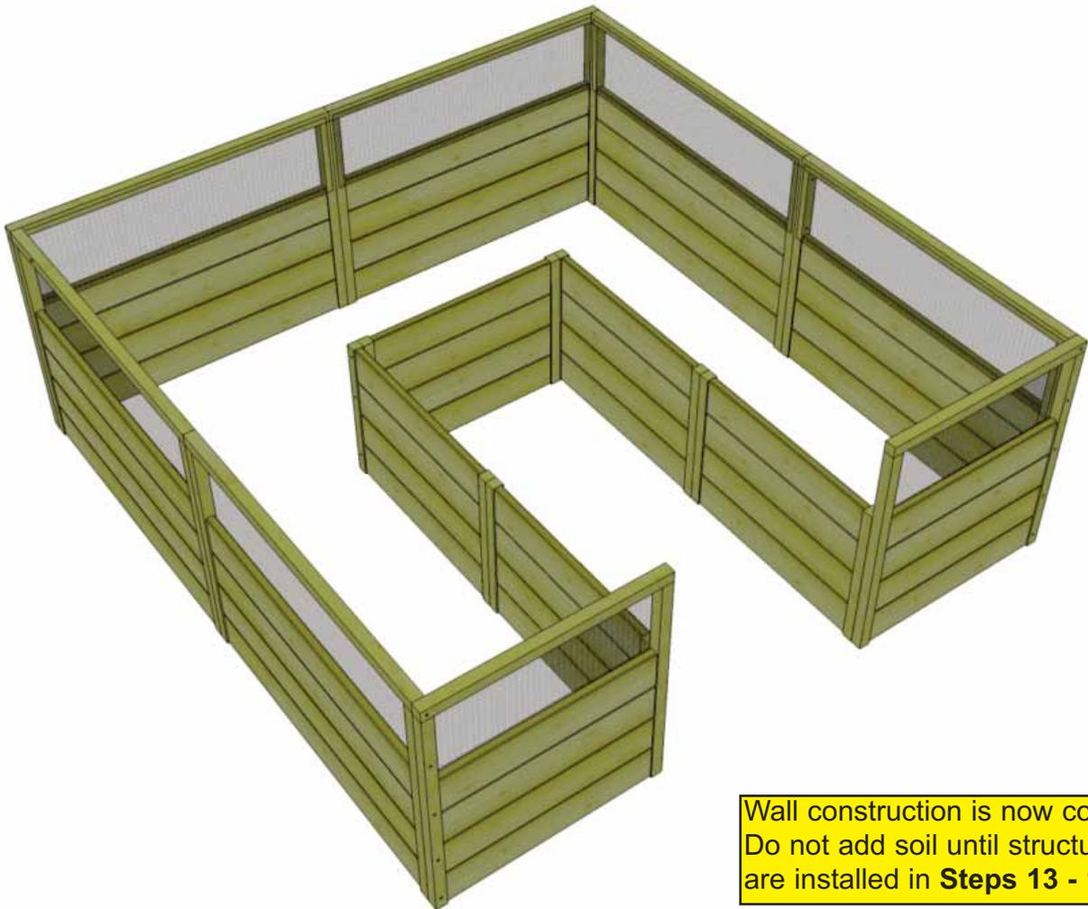
Wall construction is now complete. Do not add soil until structural ribs are installed in **Steps 13 - 17.**
