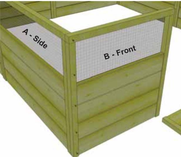
**8.** Align and attach remaining **Side Panel (Part A)** and **Front Panel (Part B)** as per **Steps 2, 3 & 4**. Attach with 5 - 2 1/2" Screws per panel.
