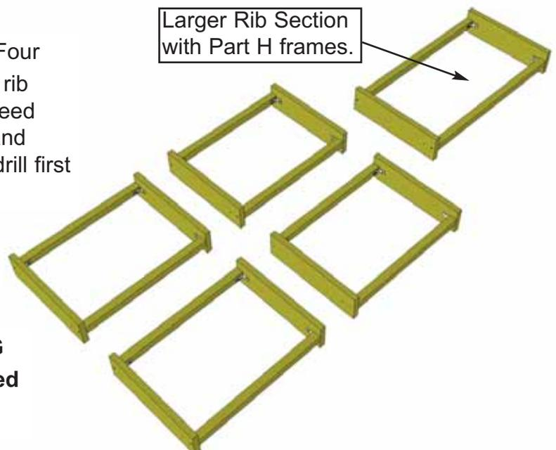
**15.** Complete 5 bed rib sections. **4** with **Part G Bed Rib Frames** (shorter) and **1** with **Part H Bed Rib Frames** (longer).
