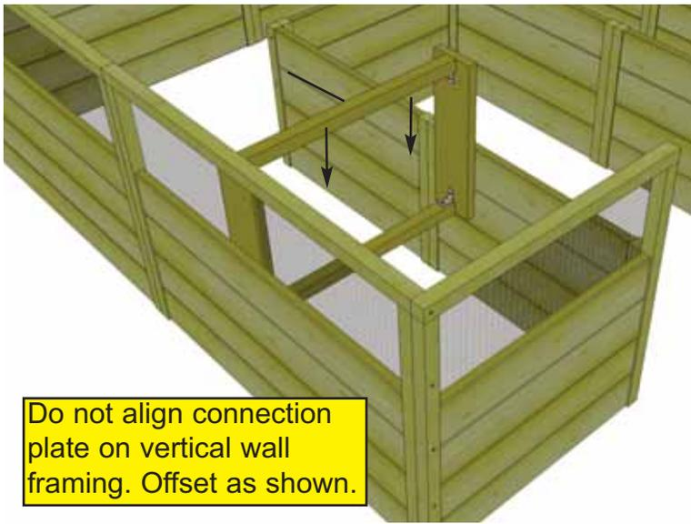
Do not align connection plate on vertical wall framing. Offset as shown.
