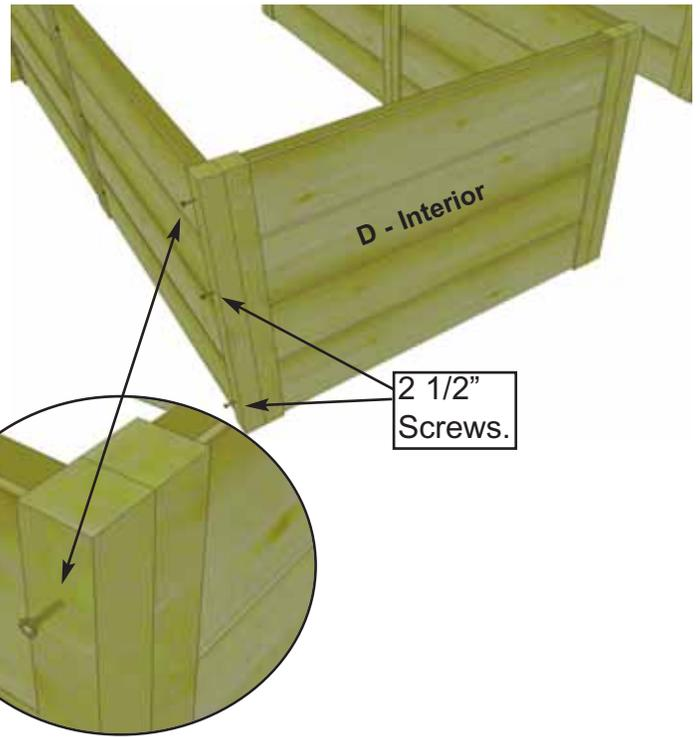
**12.** Align and attach **5th Interior Panel (Part D)** between frames of attached Interior panels. Attach with **3 - 2 1/2" Screws** per corner (6 screws in total).
