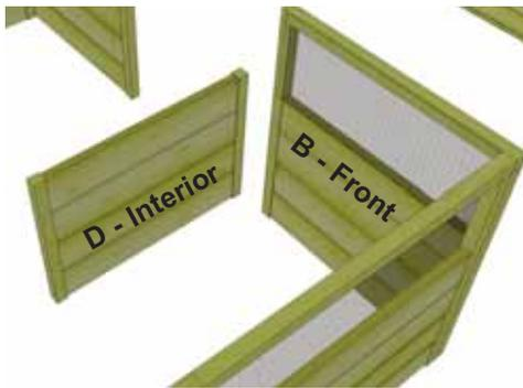
Interior Panel framing flush with Front Panel Framing.
