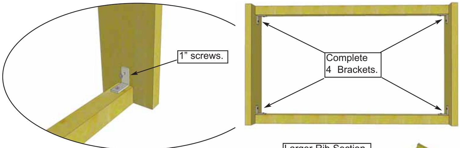
**14.** Locate "**L**" **Brackets** in hardware kit. Four brackets are required for completion of each rib section. 4 smaller and 1 larger rib sections need assembly. Position brackets in each corner and secure with **4 - 1" Screws** per bracket. Pre-drill first with 1/8" bit to prevent wood from splitting.
