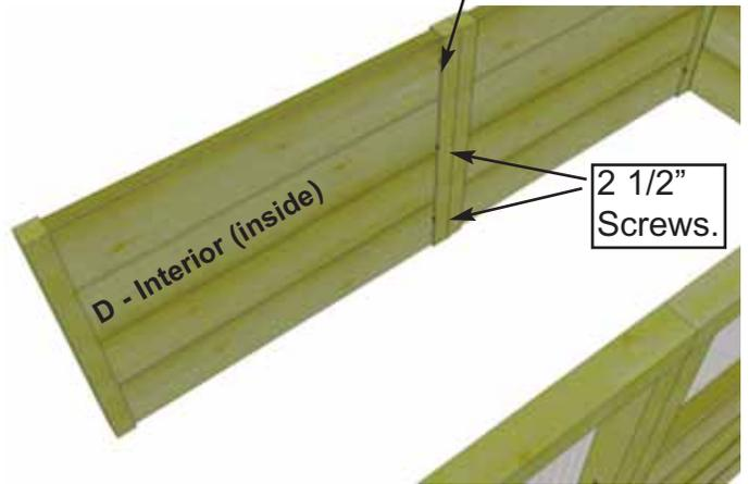
**10.** Align and attach framing of **2nd Interior Panel (Part D)** to 1st Interior panel framing. Angle screw panels together with **3 - 2 1/2" Screws** from the inside.
