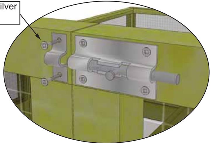
**26.** Attach **Barrel Bolt** (male and female pieces) to side framing of trellis/screen. Use **6 - 3/4" Silver screws**. Pre-drill shallow hole first to prevent wood from splitting. Do a dry run first to confirm correct position. Barrel Bolt may be silver/black.
