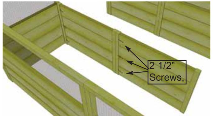
**11.** Align and attach framing of **3rd and 4th Interior Panels (Part D)** as per **Steps 9 & 10**. Angle screw panels together with **3 - 2 1/2" Screws** from the inside.
