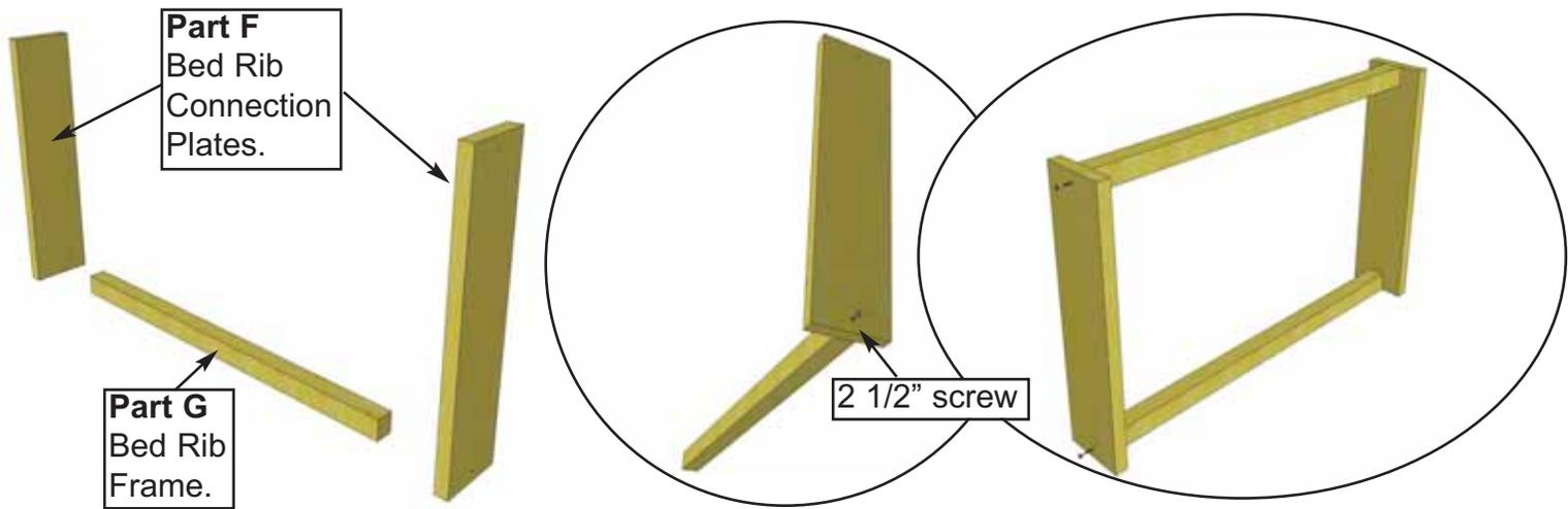
**13.** To complete rib assembly, locate all **10 Bed Rib Connection Plates (Part F) - 1" x 5 1/2" x 20"**, **8 Bed Rib Frames (Parts G) - 1 1/2" x 1 1/2" x 26 3/8"** and **2 longer Bed Rib Frames (Part H) - 1 1/2" x 1 1/2" x 29 3/4"**. On a level flat surface, screw connection plate and frame together with **1 - 2 1/2" Screw** per end. Align so plate and frame are flush at bottom. Complete both sides.
