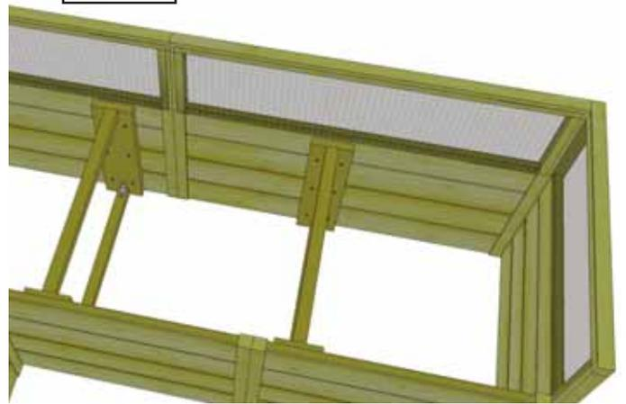
**17.** Complete remaining short **Bed Rib Frames (3)** as per **Step 16.**
