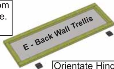
Orientate Hinge so counter sunk holes are to the outside.
