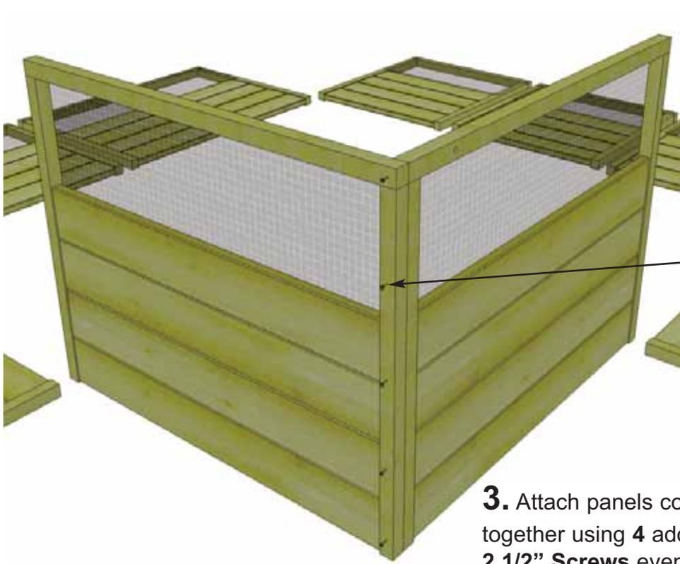
**3.** Attach panels completely together using **4 additional 2 1/2" Screws** evenly spaced on panel framing. Make sure panels are aligned prior to screwing. Pre-drill first to prevent wood from splitting.
