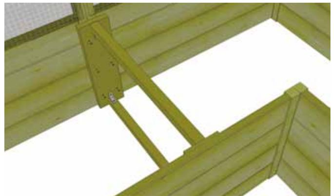
**18.** Lift and center completed longer **Bed Rib Frame** on rear and end interior panels. Align with bottom of panels. Secure with **6 - 2" Screws** per plate. **Important - Do not over screw!**
