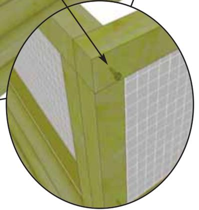
**5.** Align and attach second **Side Panel (Part A)** as per **Step 2**. Use **5 - 2 1/2" Screws** to secure.
