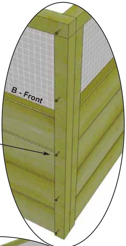
**7.** Align and attach **Front Panel (Part B)** - 30 5/8" wide to side panel with 5 - 2 1/2" Screws as per **Step 2**.
