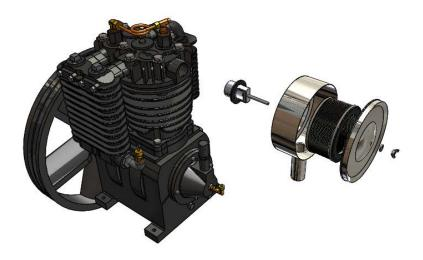
2. Install FITTING029 (1" Street L) into head intake port tighten until elbow is facing down. Install FITTING082 (barbed connector) into FITTING029 and tighten. NOTE: Standard Intake Port size is 1", however some pumps may have ½" or ¾" port sizes. Additional fittings have been supplied to reduce from 1" to ½" or ¾" if necessary. Additional components are marked (OPTIONAL) on Parts List.
