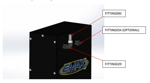
4. Place Silencer in desired location (recommend just to the left of the unit). Trim HOSE002 to desired length and slip over FITTING082 BARBED CONNECTOR.
