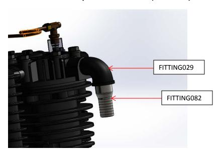
3. Install FIITING029 into port opening and tighten until elbow outlet is pointing upward. Install FITTING082 into FITTING029 and tighten. NOTE: Example shown below requires only one outlet due to a single pump filter application and addition port has been plugged using FITTING034 (1" NPT PLUG).
